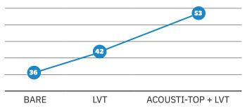
\*International Building Code (IBC) requires a minimum 50 STC/IIC (45 F-STC/F-IIC) in multifamily construction. An STC/IIC of 50 provides marginal sound control, the International Code Council (ICC), author of the IBC, recommends an "acceptable" level of performance for STC and IIC is 55 (52 if field tested). \*\*Assembly tested: 18" Open Web Truss, Insulation, Resilient Channel, 1" Underlayment
