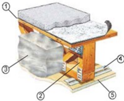
FIGURE 2 — SOUND RATED ASSEMBLY INCORPORATING WOOD TRUSSES
